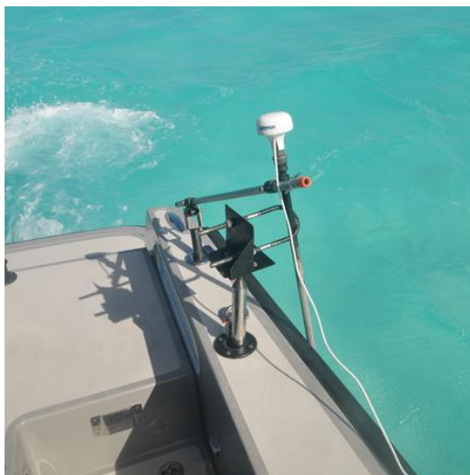
Figure 13. Photograph of GPS antenna and Depth Sounder units used for collecting data for the benthic habitat and bathymetric surveys (photo – S.Schill).
