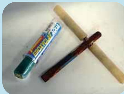
A stick of two-part epoxy putty and hand-auger made by welding a steel handle to a cold chisel and covering the handle with plastic tube (P. Cabaitan).
